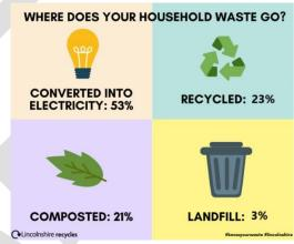
Our residual (general) waste is mainly treated and disposed of at the Energy from Waste (EfW) facility at North Hykeham reducing the dependence on landfill. The EfW became fully operational in March 2014 and can treat up to 190,000 tonnes of residual waste each year, diverting it from landfill and exporting 105,000 MWh of electricity in the process each year. In September 2019, the facility dealt with its one millionth tonne of rubbish in Lincolnshire.
